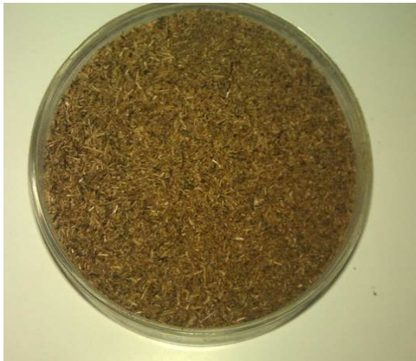
Sulphuric acid treated Sugar bagasse
