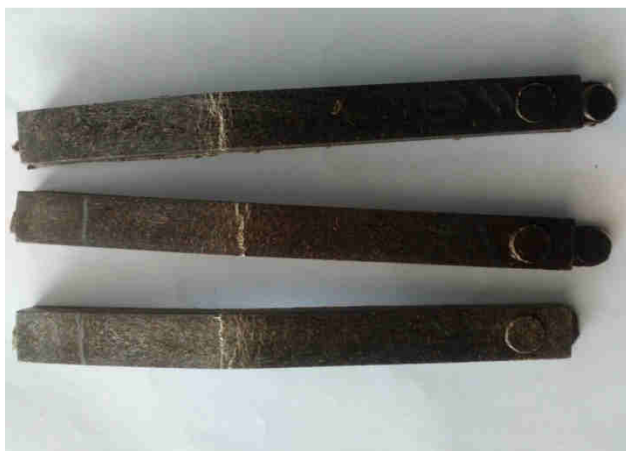
Fig.7(b): After flexural testing of composite
