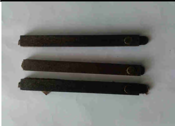
Fig.7(a): Before flexural testing of composite
