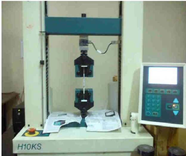
Fig .3: Loading arrangement of tensile test
