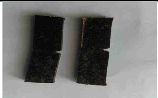
Fig.9 (a): Before impact test of composite
