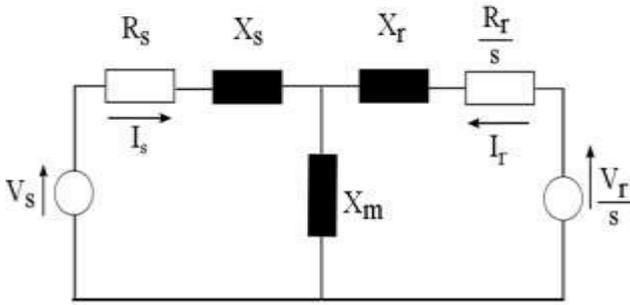
Fig. 2: Steady state T-equivalent circuit for the DFIG [2]
