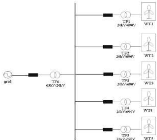
Fig. 5: An example system for simulation
