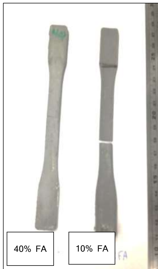
Fig.17: Separation after failure in 10 %FA-epoxy, but no separation in 40%FA-epoxy
