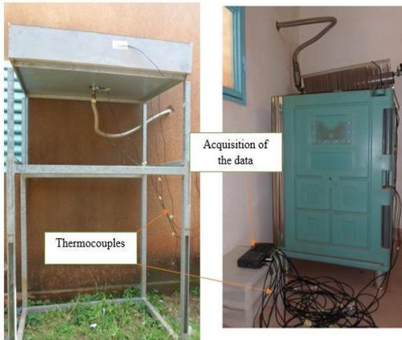
Fig.5. Acquisition of experimental data.
