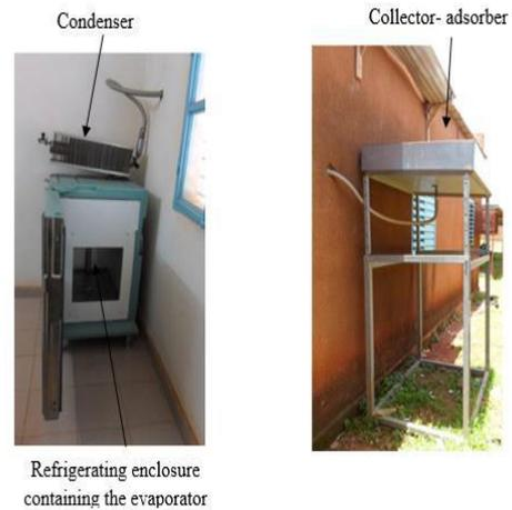
Fig. 2. Photography of solar adsorption refrigerator
