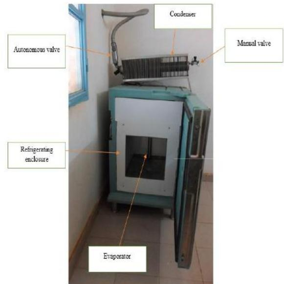
Fig.4. Detailed photograph of the condenser and the refrigerating enclosure
