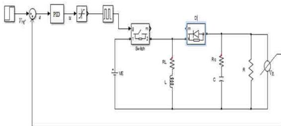
Fig. 2: The PID controller for Buck-Boost converter
