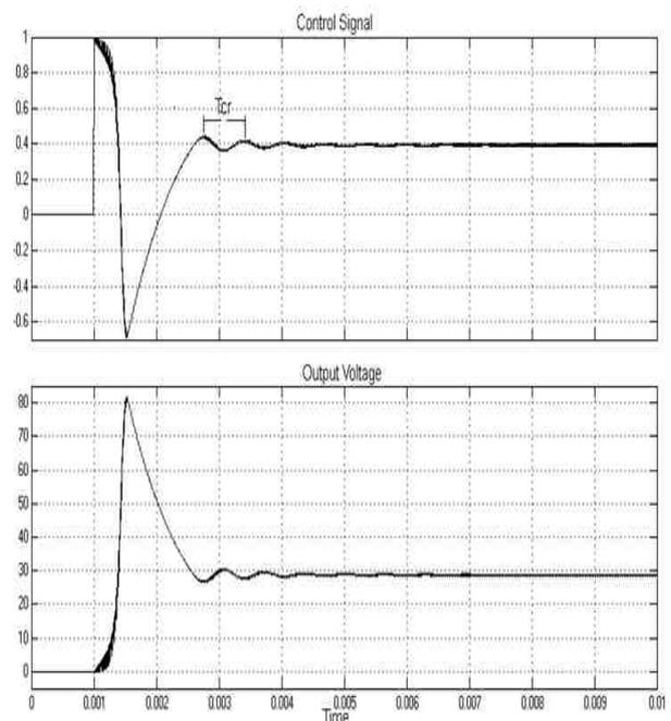
Fig. 5: Step response of the buck-boost converter with subcritical proportional gain.
