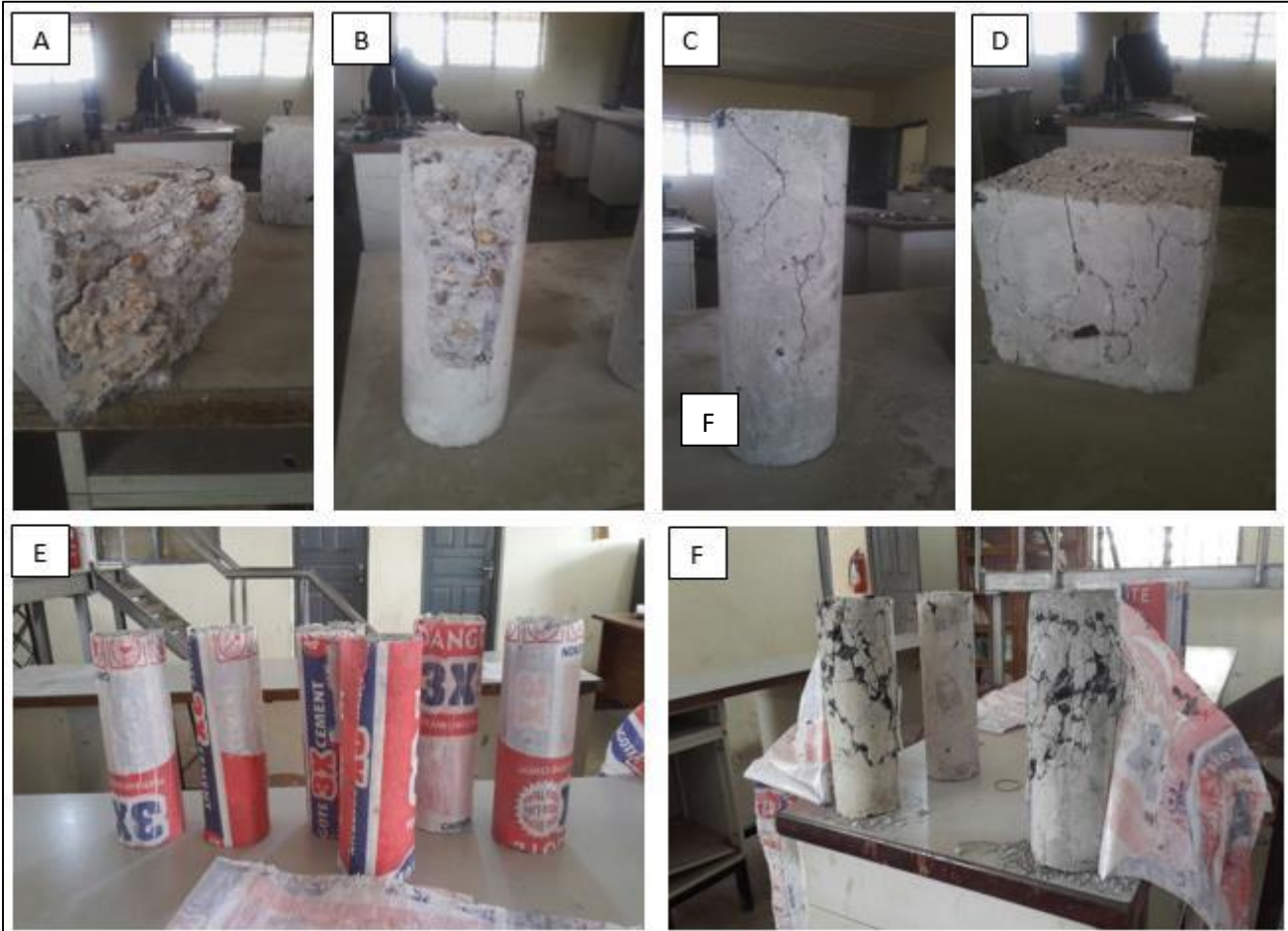
Plate 2.1: (A) Brittle failure of control cube (B) Brittle failure of control cylinder (C) Ductile failure of unconfined rubberized concrete cylinder (D) Ductile failure of rubberised concrete (E) Waste cement sack confinement of rubberised concrete cylinders (F) Ductile failure of confined rubberised concrete cylinders.
