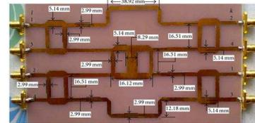
Figure 5 feeding network in hardware
