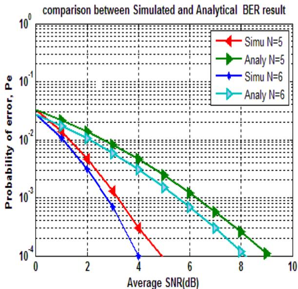
Fig.5 Analytical and simulated probability of error vs. Average SNR by varying N= 5, 6.
