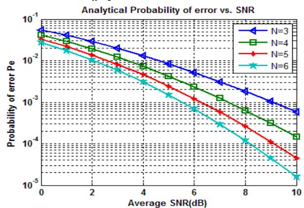
Fig.3. Analytical  $P_e$  vs. average SNR by varying no. f antennas
