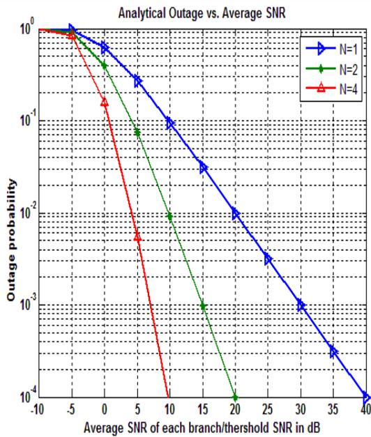
Fig.1. Outage probability vs. Average SNR by varying number of receiver antennas for N = 1, 2, 4.
