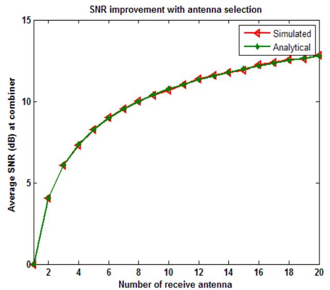
Fig.2. Average SNR at receiver vs. Number of receive antenna
