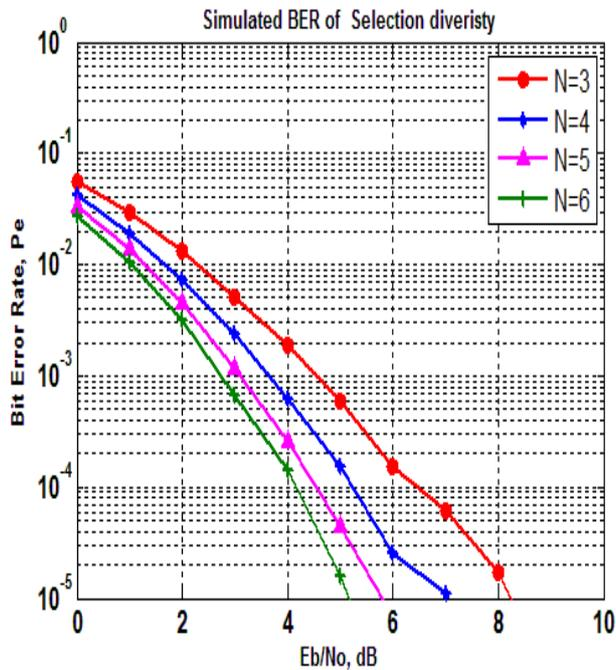
Fig.4 Simulated probability of error vs. Average SNR by varying Number of receiver antenna, N=3, 4, 5, 6
