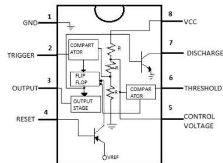
figure1: 555 Timer Block Diagram
