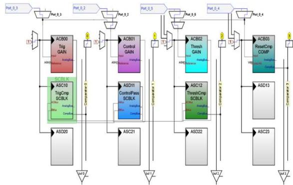
figure4. Analog block configuration on PSoC designer
