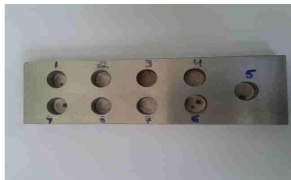
Fig 3: Work piece with blind holes after machining
