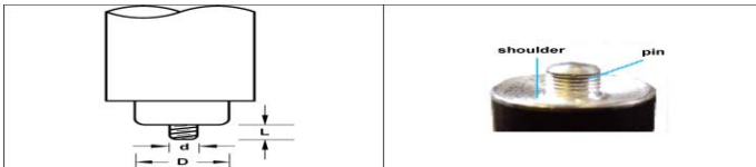
Fig (1).friction stir welding tool dimensions.
