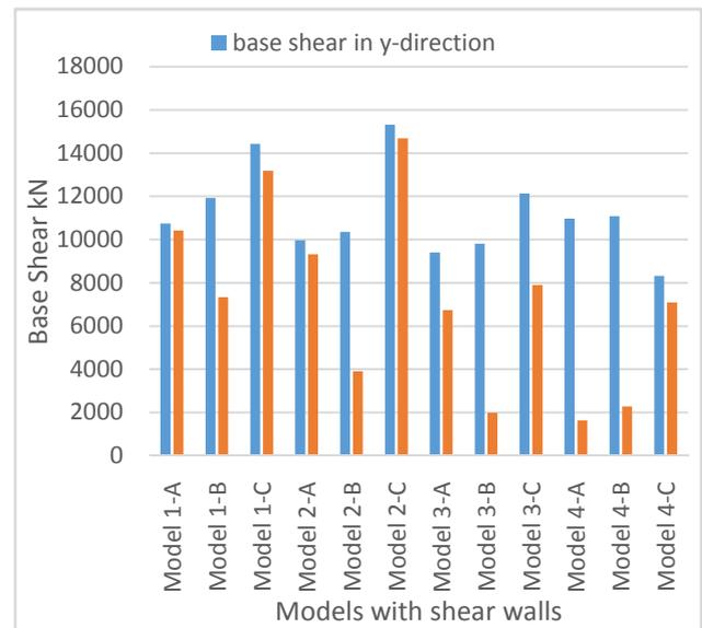
Figure 4.1.4 3 base shear variation when ground motion in x- direction in models with shear walls
