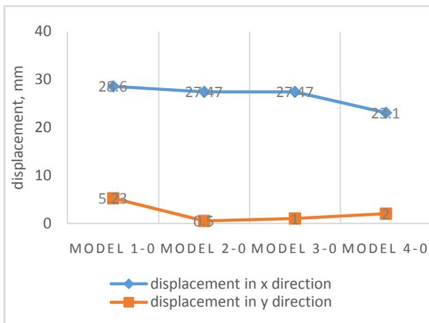
Figure 4.2.1 variation of roof displacement due to ground motion in x-direction in models without shear walls.
