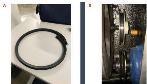
Fig. 25: The broken belt
