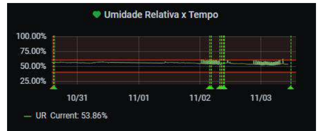
Fig. 21: Humidity from 10/30/2020 to 11/03/2020 in the air conditioning duct outlet
