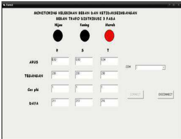
Fig.7. Visual Interface when Overload
