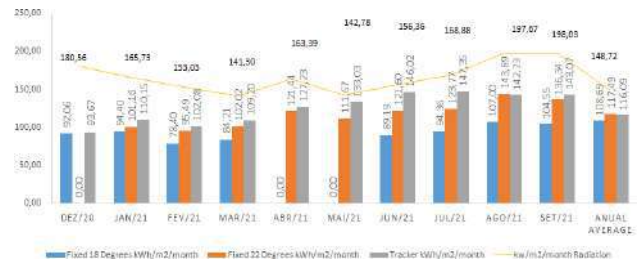
Fig. 7. Monthly energy production of each system and in-plane irradiation.
