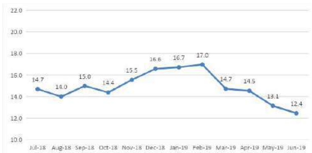
Fig. 15: History of the average wheel change time excluding the impact of unavailability of new wheels (min).
