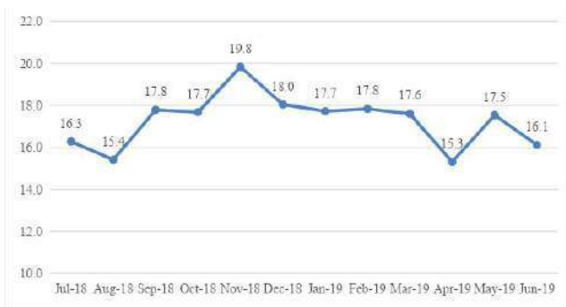
Fig. 13: History of the average wheel change time of the control group (min).
