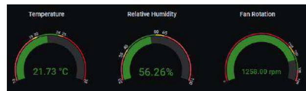
Fig. 8: Represents temperature, relative humidity and rotation instantaneous reading
