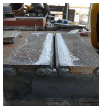
Fig.6: GTAW groove test weld assembly to allow welding with and without purging gas.
