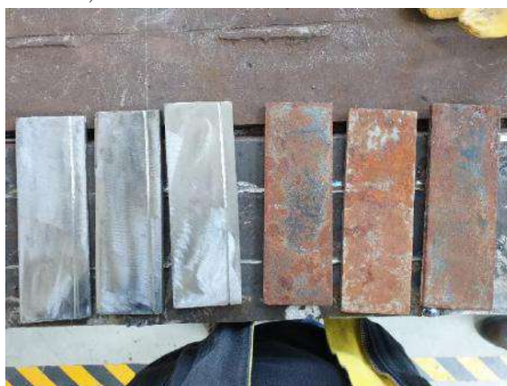
Fig.5: Bright polished and rusty plates of ASTM A36 150 X 50 X 8 mm
