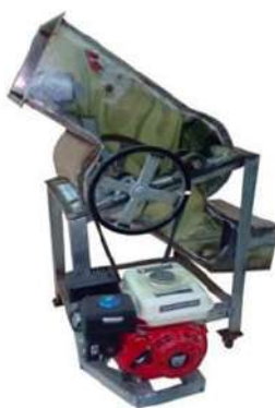
Fig.2: The result of the design of a block ice crusher using a double crusher system
