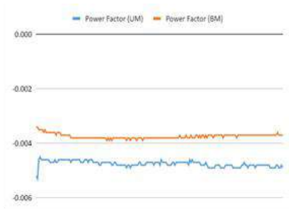
Fig 6. Comparative graph of the power factor of the System in Utility Model and in Back-up Mode using the datalogger
