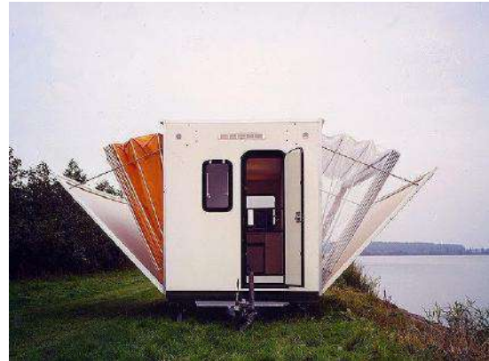
Fig.3 - Trailer designed by Böhlingk with sides being mounted
