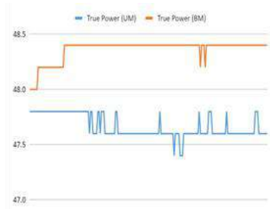
Fig 5. Comparative graph of the true power of the System in Utility Model and in Back-up Mode using the datalogger
