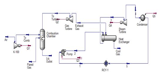
Fig.2. The Aspen Hysys Simulation Case of Combined Gas-Steam Plant
