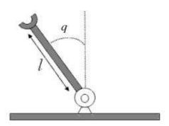
Fig. 3: One link robot manipulator
