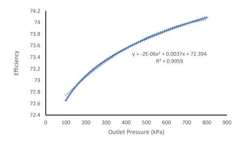
Fig.7. The Profile Plot of Polytropic Efficiency of Steam Turbine versus Outlet Pressure of Turbine
