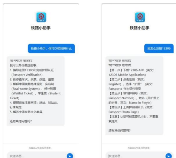
Fig. 7: Railway Assistant test transcripts: (left) function-overview response listing the agent's five core capabilities; (right) registration-guidance response decomposing the process into four steps with English glosses.
