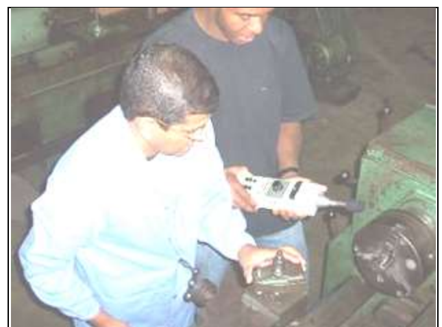
Fig. 5: Measuring the noise level of the lathe.
