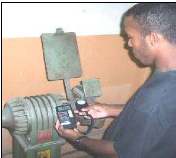
Fig. 6: Measuring the brightness near the grinder
