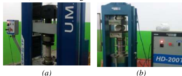
Fig.4: Mechanical tests: (a) axial compression, (b) diametral compression traction.
