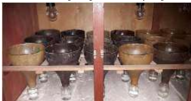
Figure 3 - Mesofauna extraction apparatus from soil samples by the Berlese-Tullgren funnel method.
