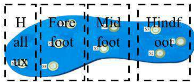
Fig.2 –Insole, on the right foot, mounted with 9 piezoresistive sensors (s1, s2, s3, s4, s5, s6, s7, s8, s9), for testing.
