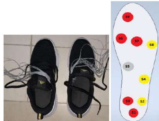
Fig. 10. 36 insoles in sneakers and illustration of pronated stepping
