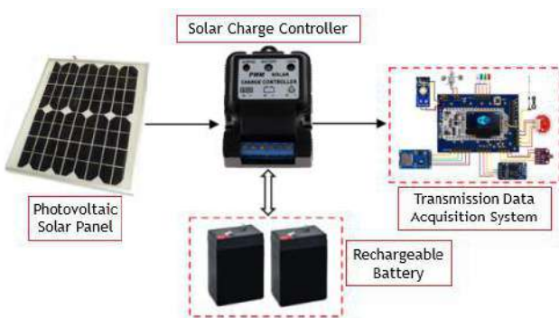
Fig. 5 Load controller system architecture.
