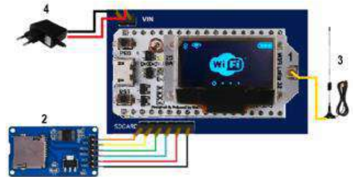
Fig. 6 Structure system of the DAS_R. (1) LoRa 32 V2 WiFi board; (2) MicroSD module card; (3) Antenna LoRa 868 MHz - 915 MHz and (4) 5V power supply.
