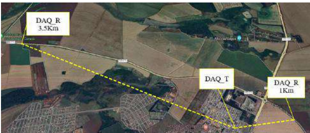
Fig. 10 Communication distance between systems with original antenna and TX900 antenna.
