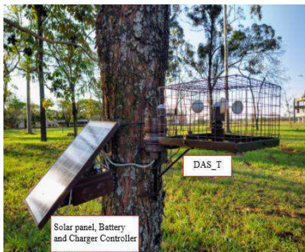
Fig. 14 Final structure system DAS_T.
