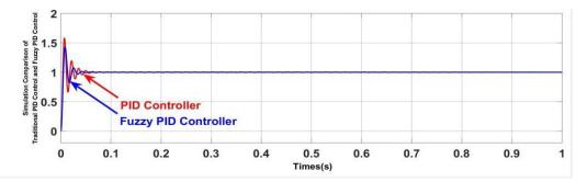
Fig.9 Response Curves of Traditional PID and Fuzzy PID Controller Systems (Swing Angle)
