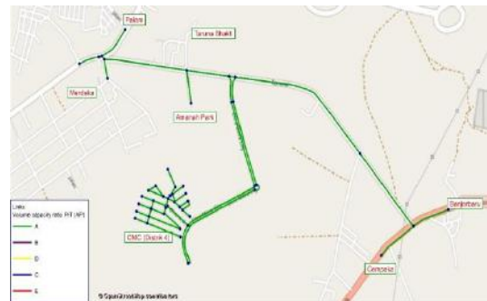
Fig.10: The LOS Simulation and the Amount of the Traffic Flow of the Road Section of Post-development at Peak Hour
