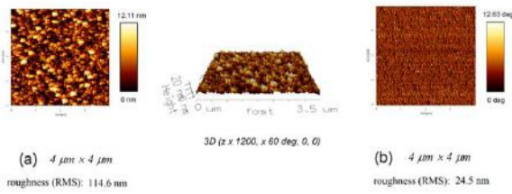
Fig.4: AFM of thin film. (a) 4 × 4 μm images of the height (topography profile) and (b) 4 × 4 μm lock-in phase image.
