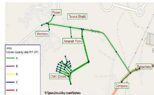
Fig.11: The LOS Simulation and the Amount of the Traffic Flow of the Road Section of the 5-year Post-development at Peak Hour
