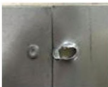
Fig.24: Failure mode of SPR connections.
