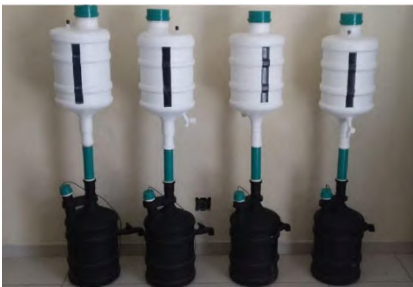
Fig. 5: Constructed Prototypes of Biodigesters Source: Produced by the author (2021)
