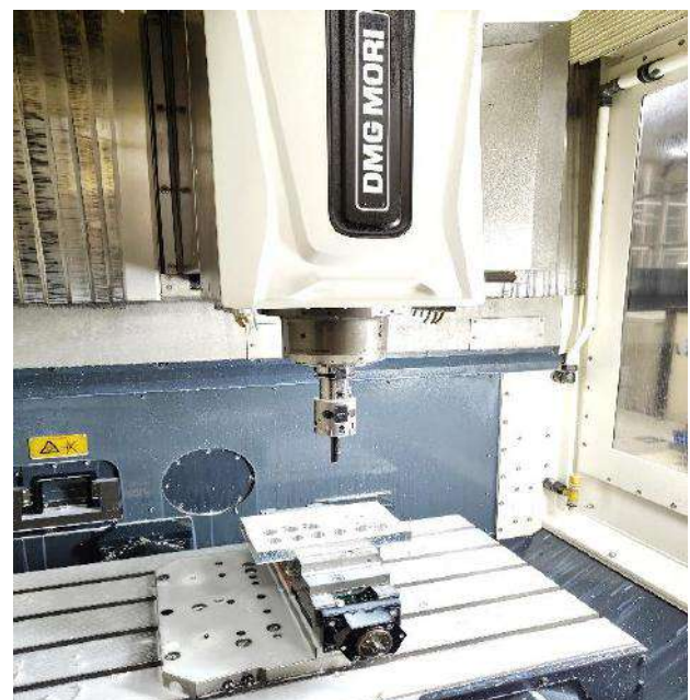
Figure.1 : Boring operation on 3-Axis CNC Vertical machining Centre, DMG MORI D650V
