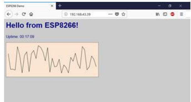
Fig. 3. NodeMCU 12e monitoring screen via WiFi site.
