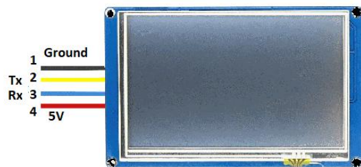
Fig. 4. The connection pins used with the display Nextion.
