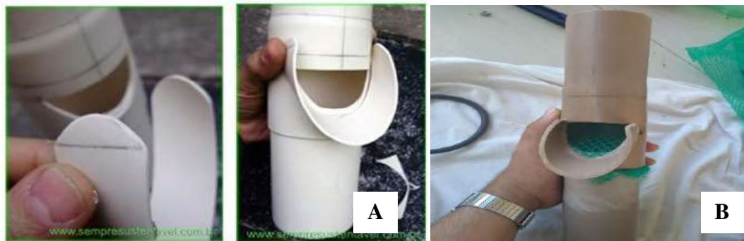
Figure 5:A - Filter nozzle construction, B - filter ready trough.
