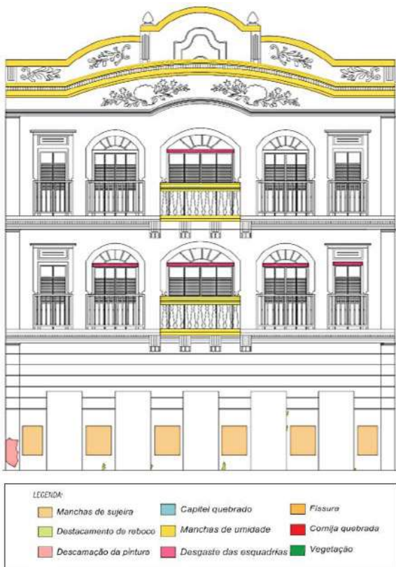
Fig. 12: Damage map of the front façade
