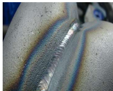
Fig.2: Continuous welding of exhaust system pipe.
