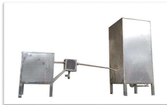
Fig.2: Pyrolyzers with multilevel condensation system
