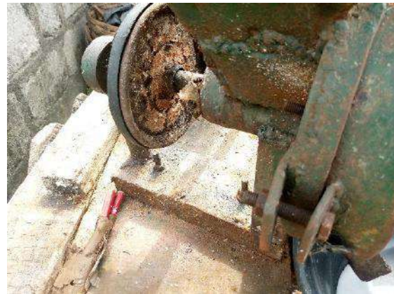
Fig 1 mild steel exposed to tomato fluid.
