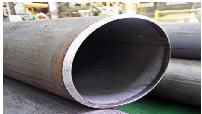
Fig 9. Cement Mortar Lining
