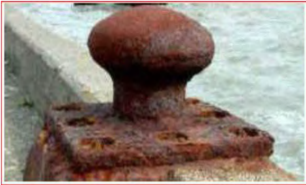
Fig 2. Uniform Corrosion (Mgonja, 2018)
