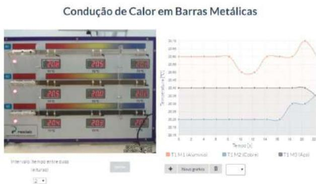
Fig. 2: LR Heat conduction in metal bars
