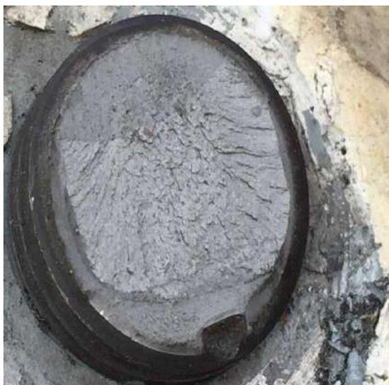
Fig. 3-13: M33 high strength bolts fracture
