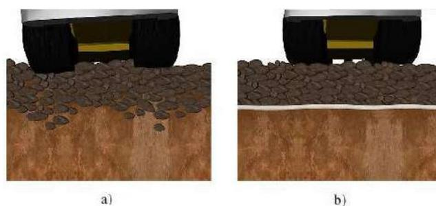
Fig.3: Simulation of geosynthetic application
