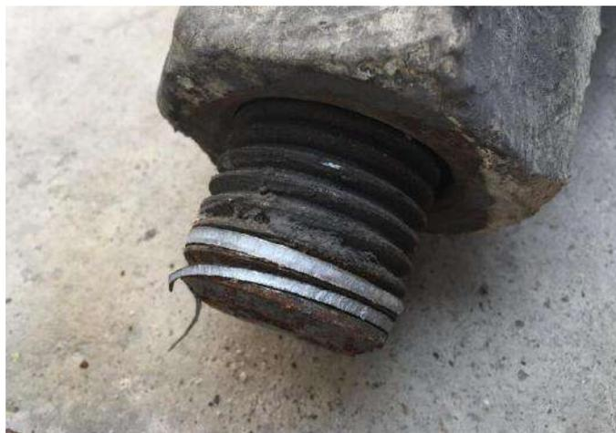
Fig. 3-9 M42 high-strength bolt out of the thread
