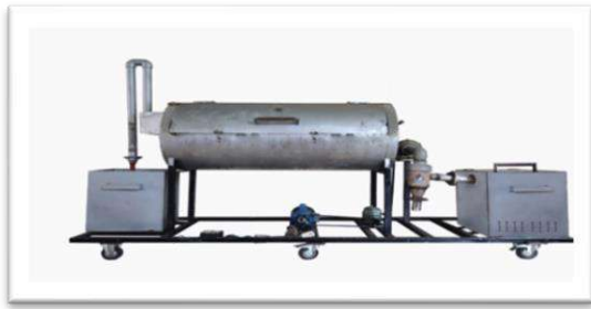
Fig.2: Fish Smoking Equipment with Smoke Filtration Using Cyclone Separator.
