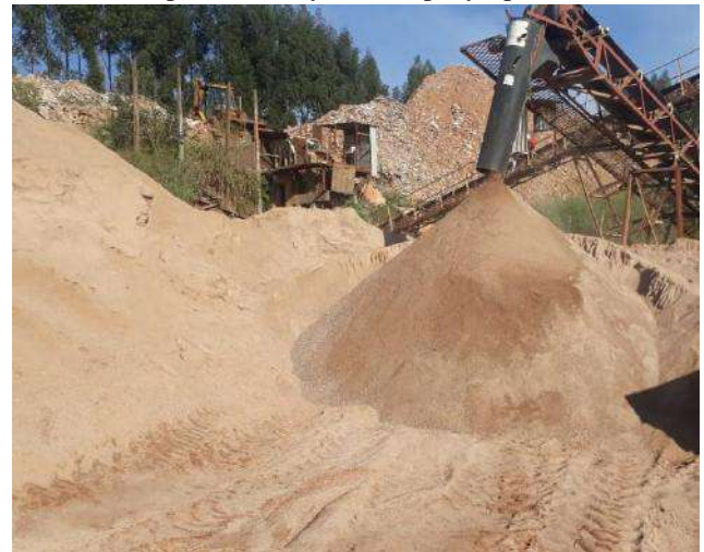
Fig. 1: Aggregates recycled at FUTURE (Author)
