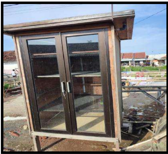
Fig.2 Results of the design of the fish dryer
