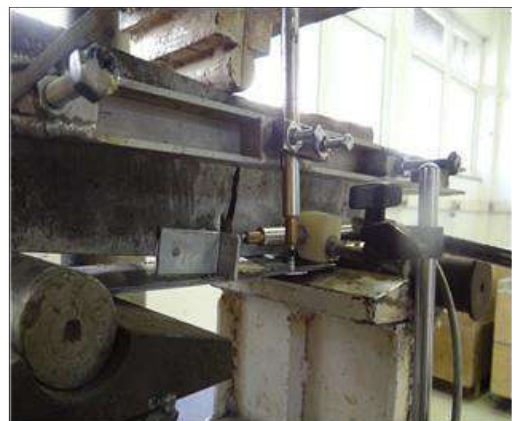
Fig. 3: LVDTs to measure \omega and \delta .
