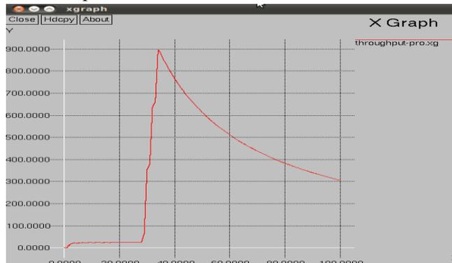
Fig.3: Throughput of CC-BTS Topology without compression
