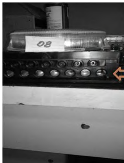
Fig. 1. Illustrative image of the ME 2, highlighting the region of easy access of the internal electronic circuit, with the use of drill.
