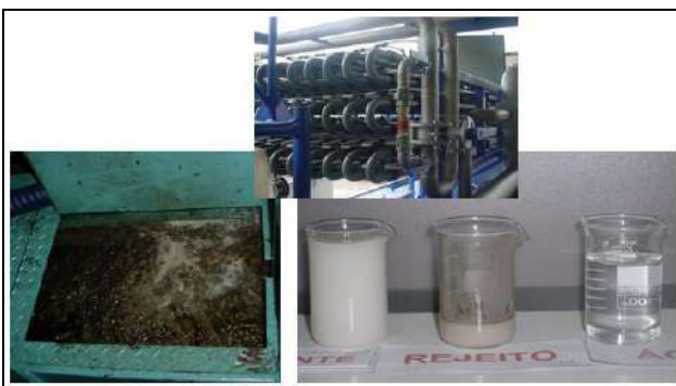
Fig. 9: Result of centrifugation followed by ultrafiltration
