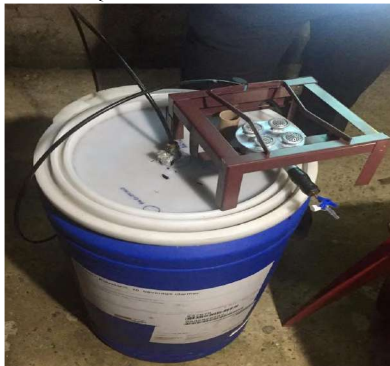
Fig.2: Single-stage reactor with a capacity of 70 liters
