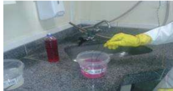
Fig. 5: Test piece being emerged in the container containing degreaser
