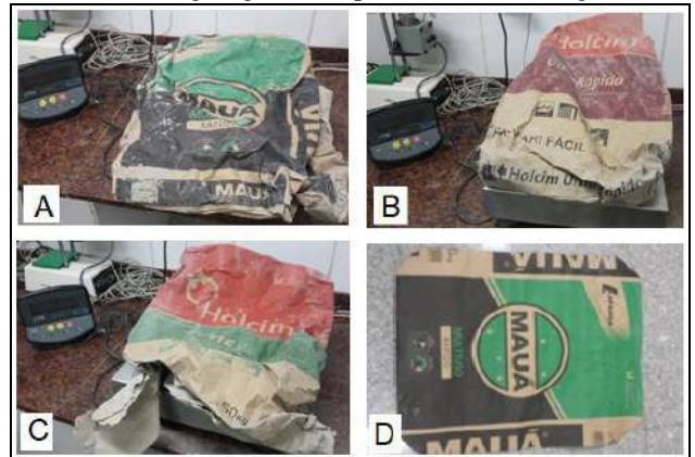
Fig. 2 - A, B and C samples of post-consumer packaging and D unused packaging
