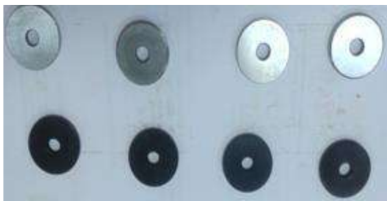
Fig. 10: Before and after black oxidation - test pieces
