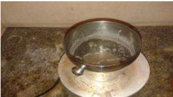
Fig. 7: Black oxidation test by RQ - OXID FE
