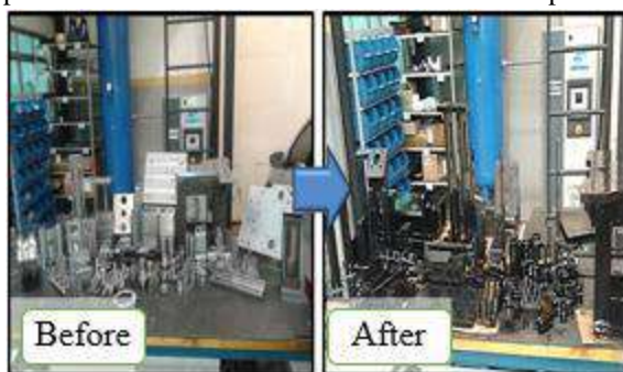
Fig. 11: Before and after black oxidation - Production
