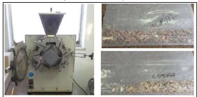
Fig. 3 - Knife mill and samples after grinding and a reduced sample.
