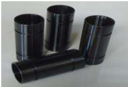
Fig. 2: Parts after layer conversion (black oxidation)[9].
