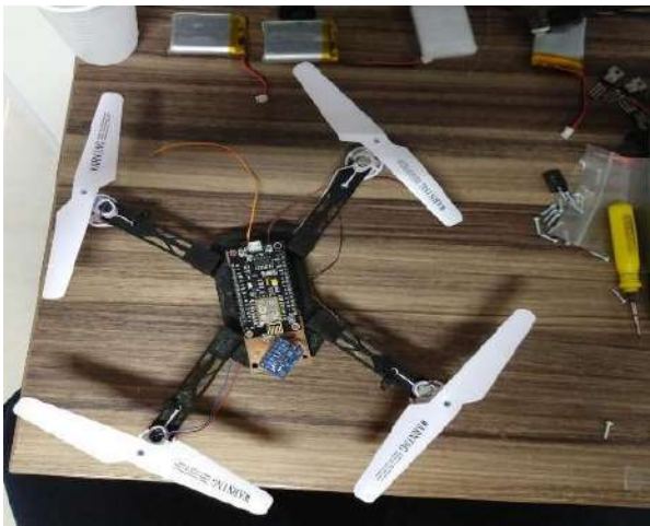
Fig. 3: Drone's parts printed in 3D
