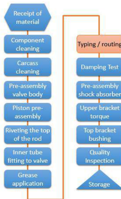
Fig. 1: Flowchart of the damper assembly process
