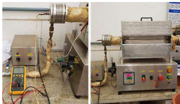
Fig.2: Fixed bed reactor in stainless steel body.
