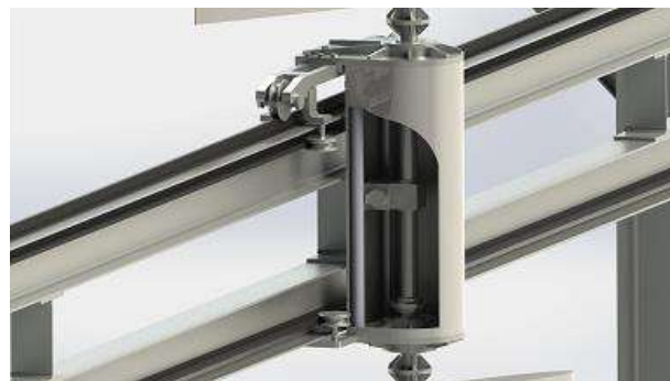
Fig. 9: Trolley and the track structure of the super turbine
