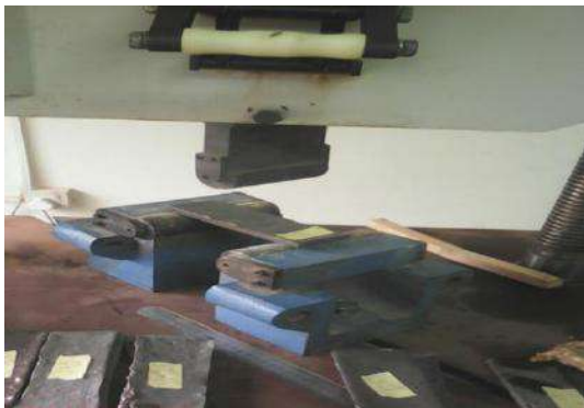
Plate 7: Flexural Test of WPC
