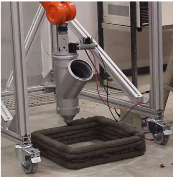
Fig. 3: An experiment of 3D printing of Concrete.
