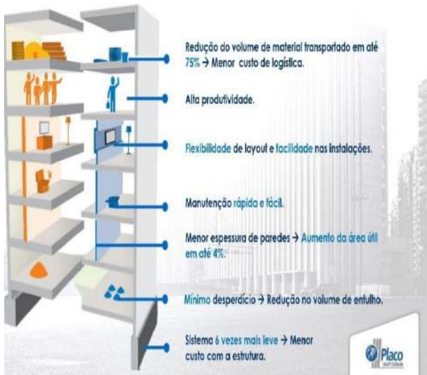
Fig. 3: Comparison of Masonry x Drywall Construction System
