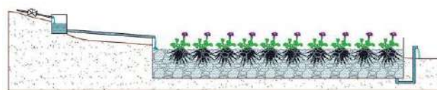
Fig.3 – Longitudinal cutting of a cultivated subsurface flow bed with Eichhornia crassipes
