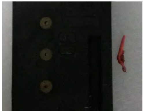
Fig.4 - extravasated filling material removed
