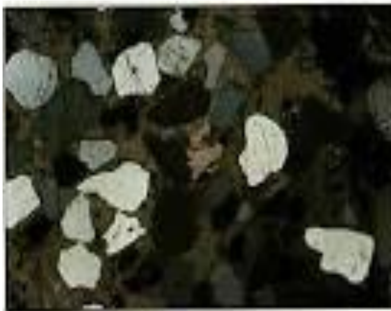
Plate 2 Photomicrograph showing Basalt under cross polarized light (Magnification x 100)
