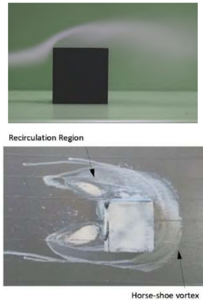
Fig. 23: Visualization of the flow over a square cylinder surface mounted.
