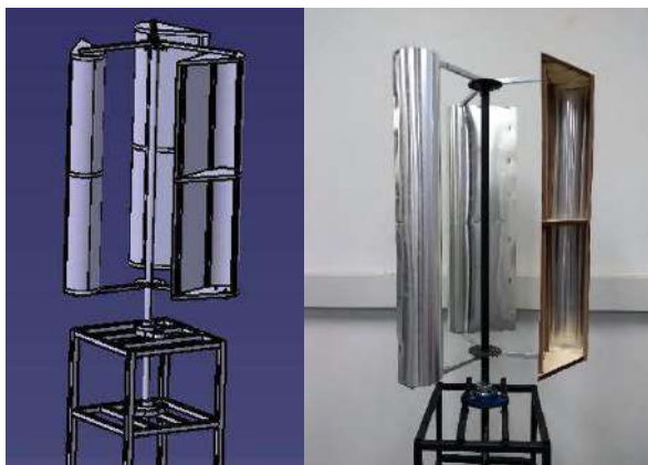
Fig. 26: 3D-drawing and photo of the Lenz-type VAWT.
