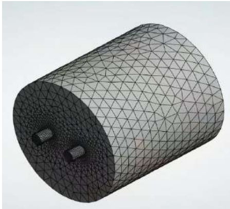
Fig.2: Mesh generation and independence verification of the fluid domain in the piston expander
