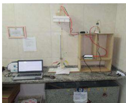
Fig.2 - Langendorff system used to study heart in vitro of control and PTU treated rats. Source: Authors, 2018.
