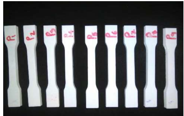
Fig.3: Parts fabricated by FDM machine
