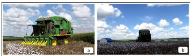
Fig.5: Self-propelled picker and the cotton drum wrapped in polyethylene film
