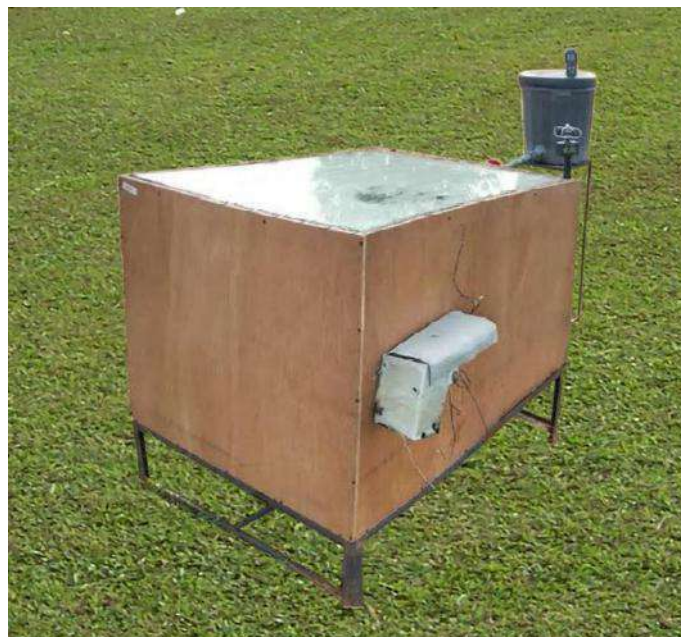
Fig.2: Experimental setup of the double effect solar still with a paraffin wax underneath absorber
