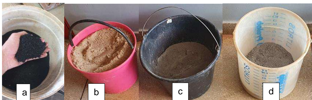
Fig.1: (a) crushed rubber, (b) sand, (c) gravel powder, (d) Portland cement.
