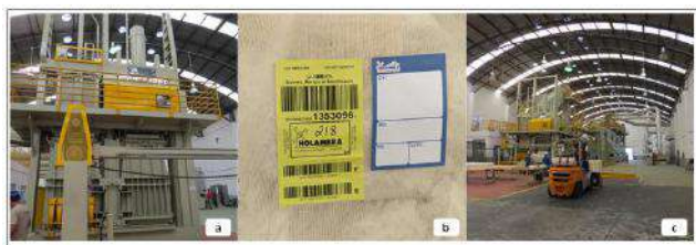
Fig.9: Smart Box 45 press, bale labeling and transport to storage
