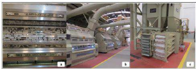
Fig.8: Ginning, lint cleaning and fibril pressing
