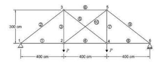
Fig. 9: Structural scheme of the flat truss (Li e Zhang [14])
