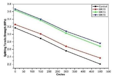
Fig. 3: Splitting tensile strength at various exposure durations
