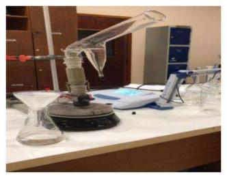
Fig. 7: Modified Hallimond tube of the laboratory type
