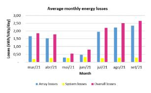
Fig. 5: the relative losses of the GCPVS
