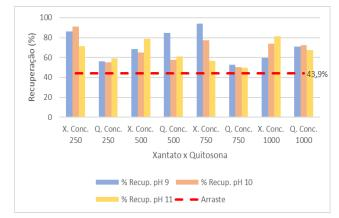
Fig. 13: Performance and behaviour of xanthate compared to chitosan
