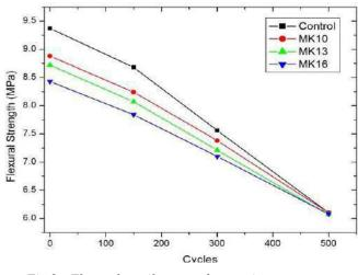
Fig.2 : Flexural tensile strength at various exposure durations
