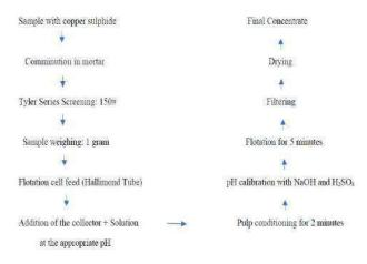
Fig. 1: Process Flowchart
