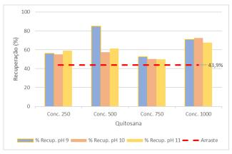
Fig. 12: Flotation test using chitosan
