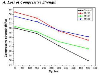
Fig.1 : Compressive strength at various exposure durations
