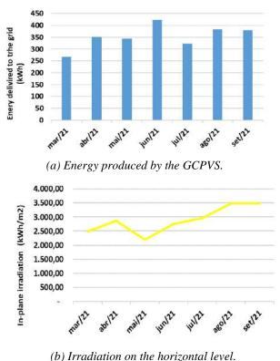
Fig. 1: Energy produced by the photovoltaic system and irradiation on the horizontal level.
