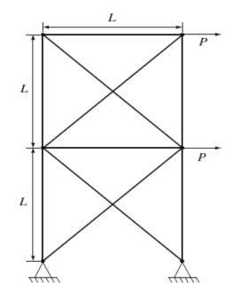
Fig. 13: 10-bar truss structure (SHAYANFAR et al. [12])
