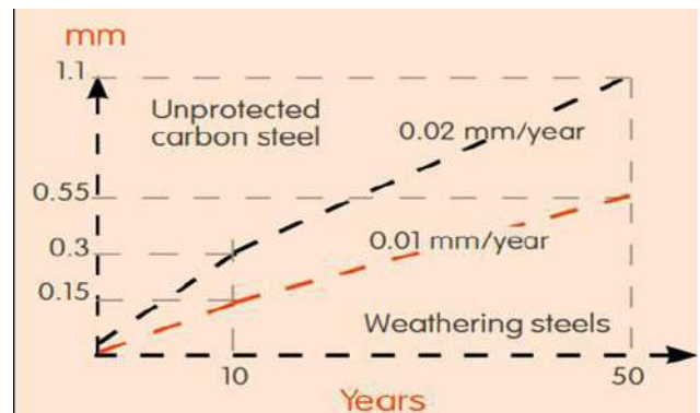
Fig.10.- Comparison of annual loss due to corrosion between carbon steel and Cor-Ten steel
