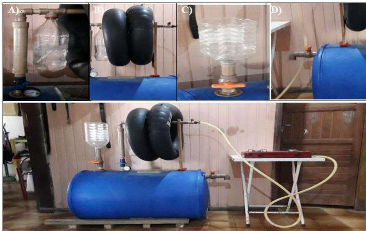
Fig.3: Adaptations made; a) two-step filter; b) gasometer; c) input; d) output; e) Complete biodigester.
