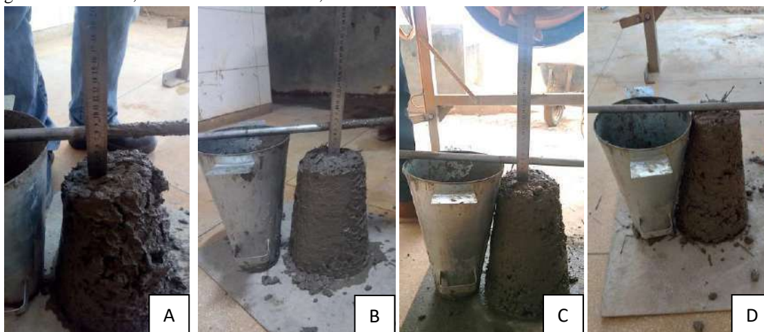
Fig.3: Cone Trunk Discharge Test, (A) Conventional Concrete, (B) Concrete with 3% Bamboo Fiber Addition, (C) Concrete with 4% Bamboo Fiber Addition, (D) Concrete with 5% added bamboo fibers.
