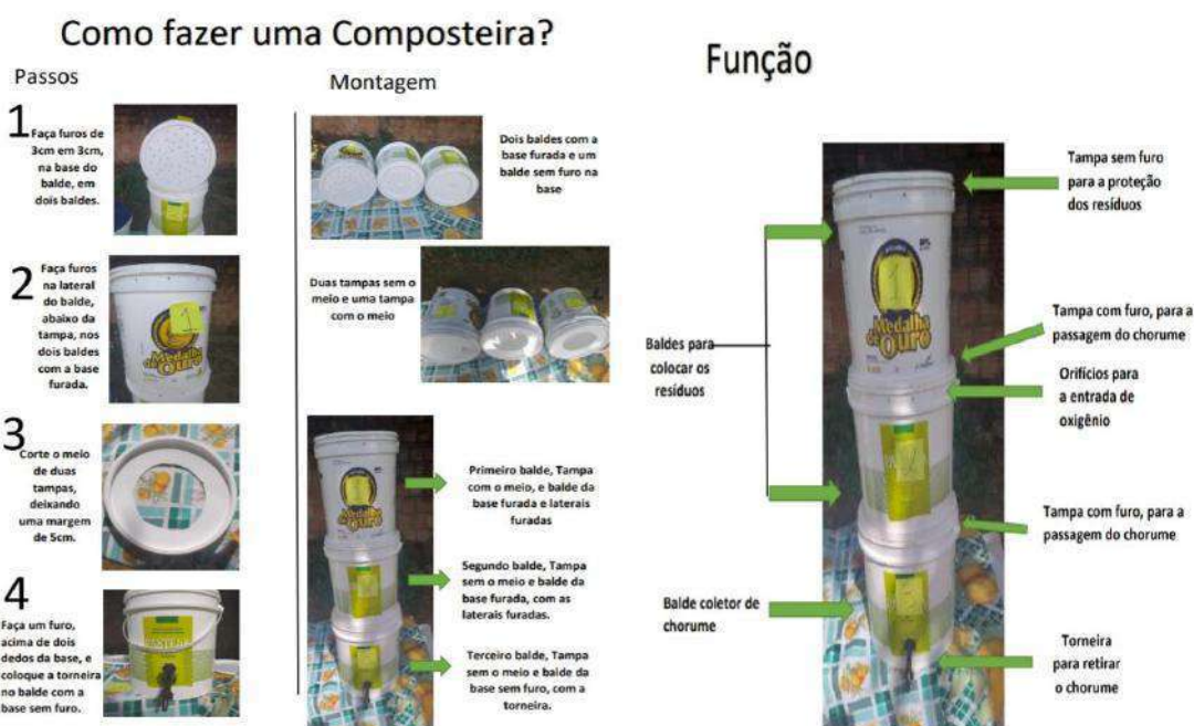
Fig.9: Primer delivered to fairs wore showing the assembly of the portable Compost separator, step by step.
