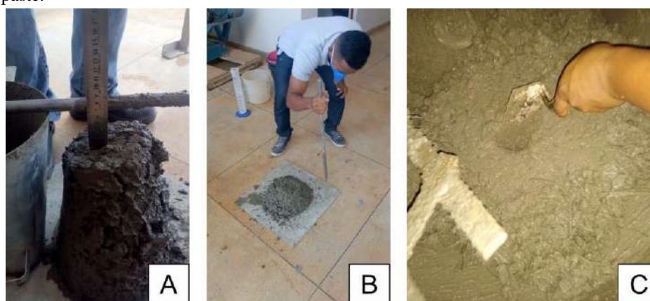
Fig.2: mixture characterization procedures, (A) Slump test performed on the trace, (B) workability verification test, (C) consistency test.
