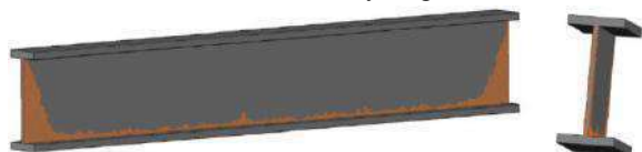
Fig 1. - Corrosion of steel beam
