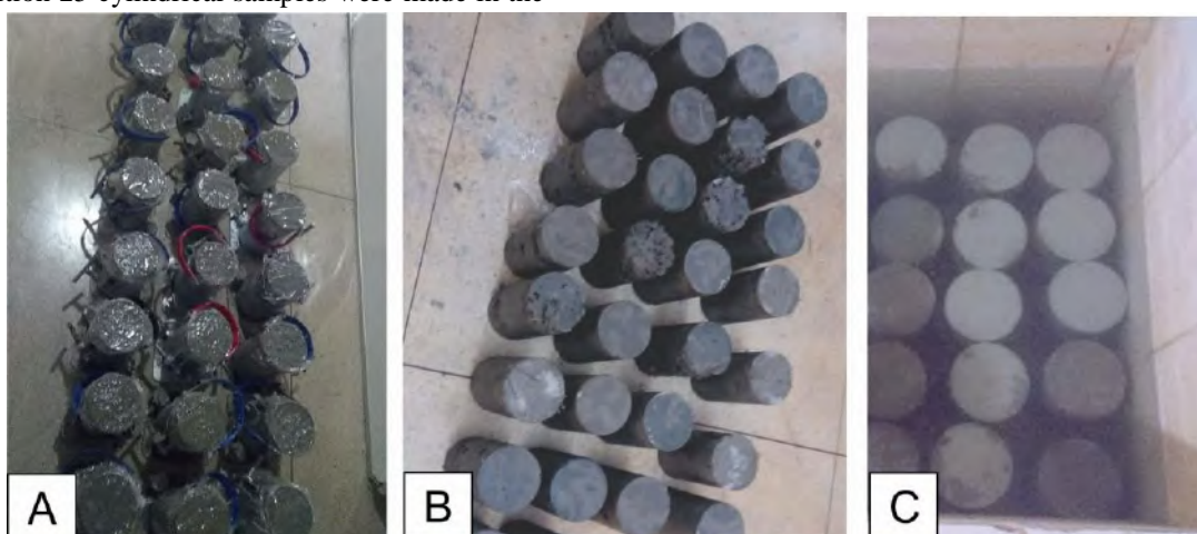
Fig.3: PC molding and demolding process (A) formation of evidence bodies, (B) removal of evidence bodies, (C) hydration and cure of bodies of evidence.
