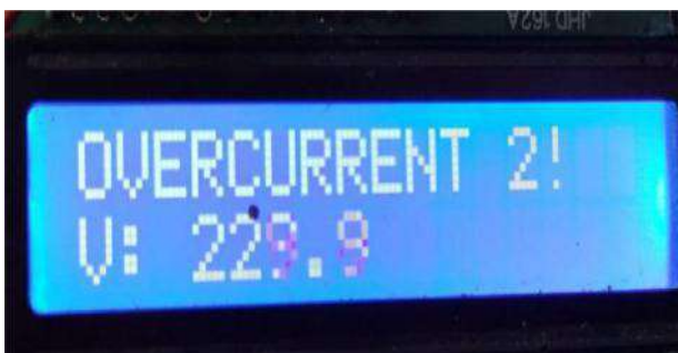
Fig.6: Result for overcurrent in Line 2
