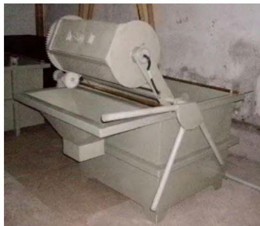
Fig. 3: Illustration of a drum electroplating machine.
