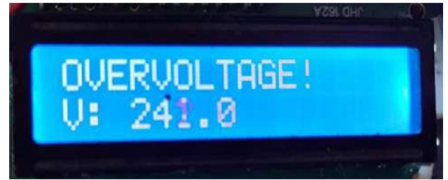
Fig.7: Result for overvoltage
