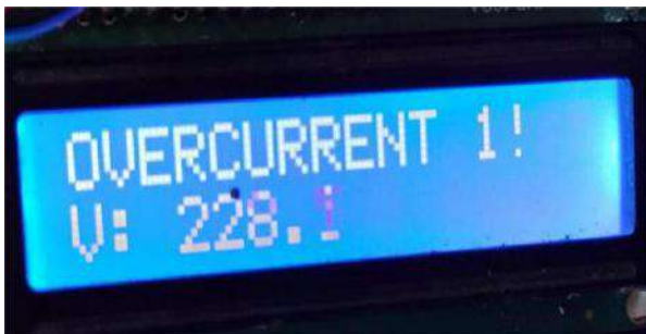
Fig.5: Result for overcurrent in Line 1
