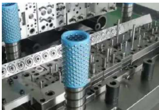
Fig. 2: Illustration of a progressive die for stamping.
