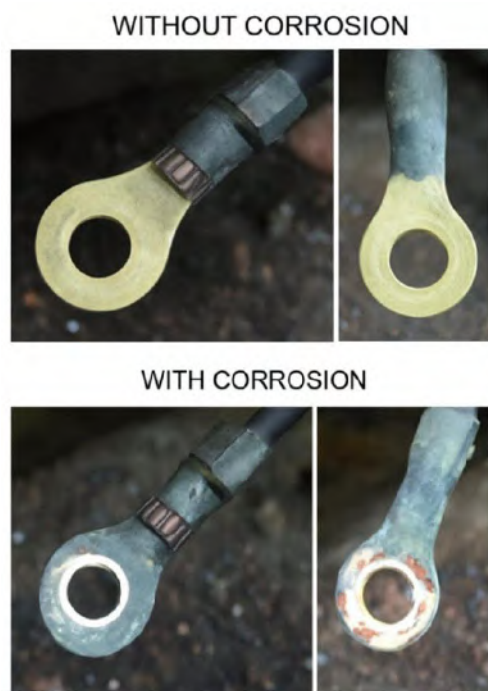
Fig. 6: Illustration of automotive grounding terminals with and without corrosion.
