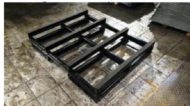
Fig.7 - Finished metal rack in AISI 1020 steel
